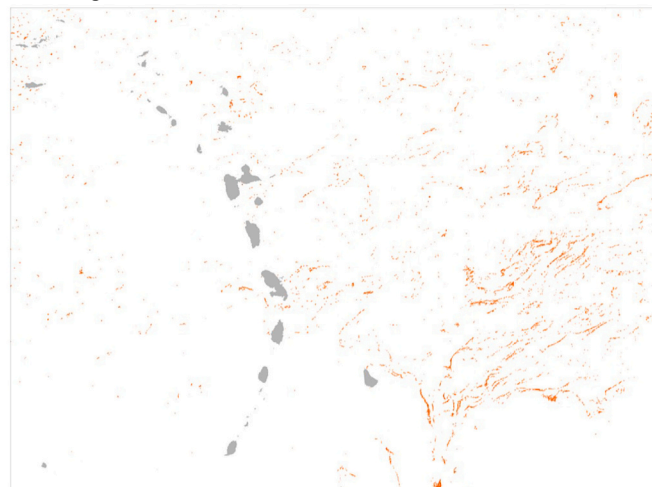
Fig. 8. Example of Sargassum detection by remote sensing in the Lesser Antilles. a: Sentinel3/OLCI satellite image from February 2, 2023; b: Masked index (Maximum Chlorophyll Index); c: Sargassum detection.
